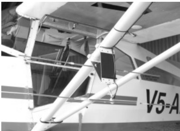
Radio-tracking aerial fitted to the wing strut of the AfriCat Maule.
